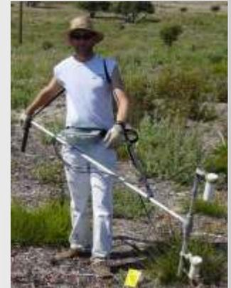
The G-858 can only detect ferrous (iron) metal. In munitions response work, most items of interest contain iron, making this an effective instrument.
