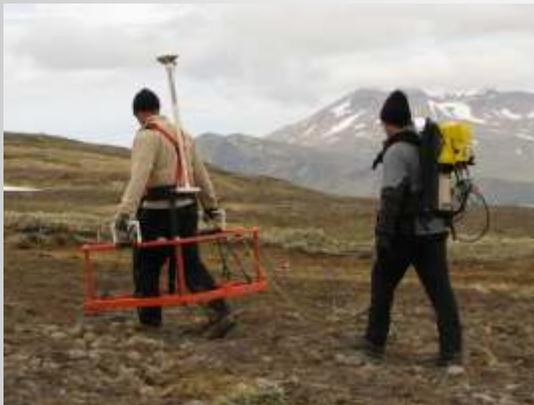
The EM61-Mark2 is usually pulled on a cart by a single operator. However, in areas with rocky terrain, like some of those around Camp Williams, this instrument is more effective when “worn” by the operator.
