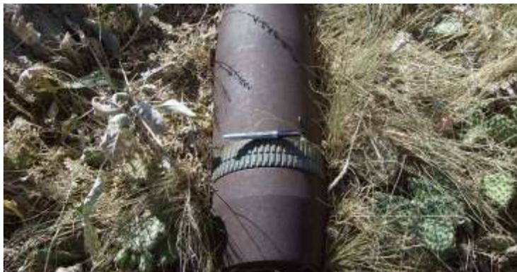
The green band around this artillery shell is called a rotating band. Protective covers were placed around the rotating bands to protect them during transport.
