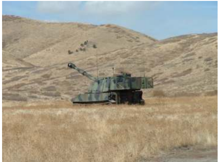
The M109A6 Paladin, a self-propelled 155mm howitzer preparing to fire.
